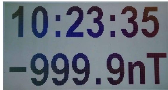
Figure 13: The main screen limits the display to +/-999nT and starts blinking from +/-600nT
