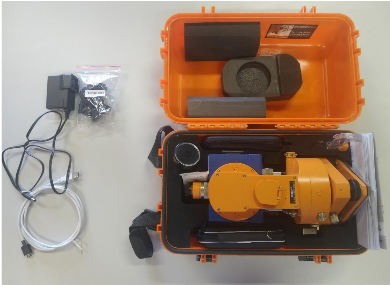
Figure 3 WiDIF DIFlux in its carrying case
