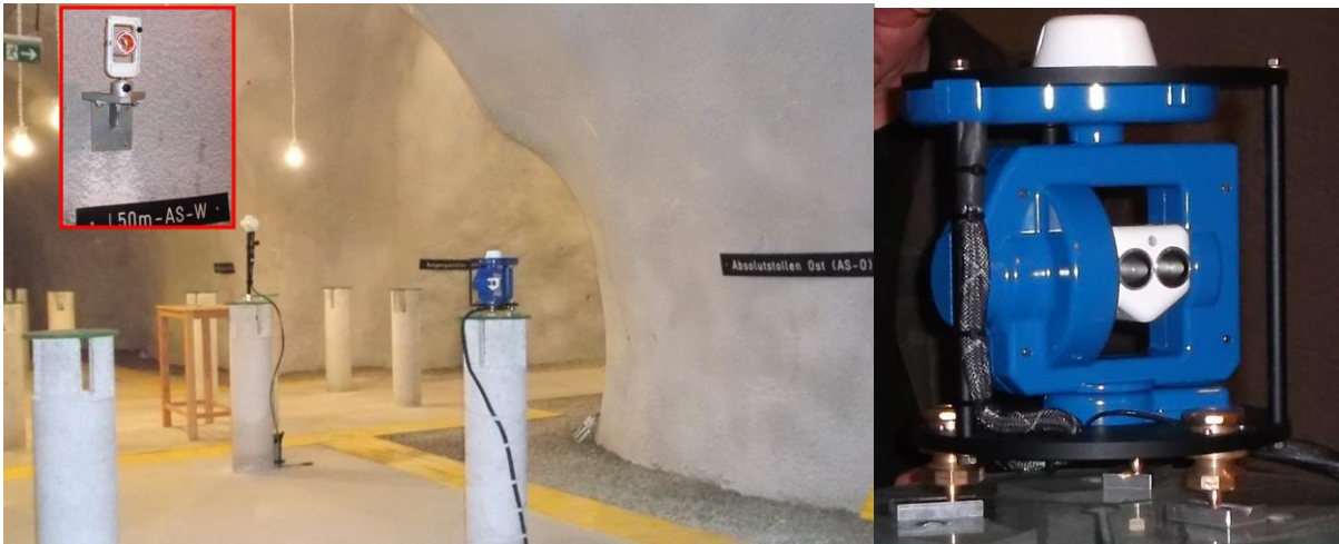
Figure 1: AutoDIF MKII installed at Conrad Observatory (WIC - Austria)
